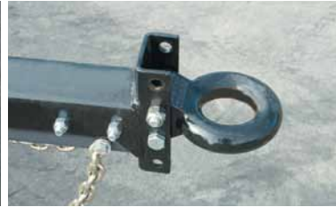
Pintle Hitch Interchanges and replaces standard ball coupler.
