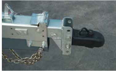
Surge Brakes Heavy-duty actuator with adjustable coupler.
