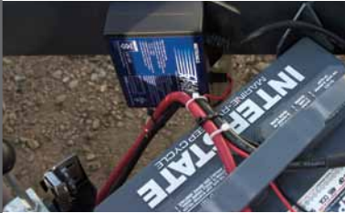
Trickle Charger 1.5-amp on-board charger with indicator lights.
