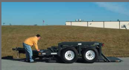
Lower entire deck to ground level
